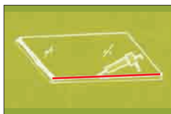
1. Place back glass on a plain surface and apply silicon sealant
