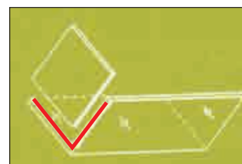
3. Apply sealant on bottom and back glass panels and fix the side glass panel
